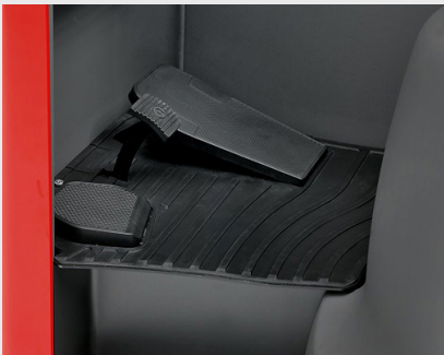
Power height-adjustable foot platform
