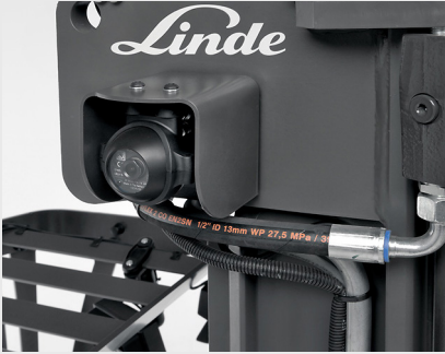
Side camera for safe transverse travel in reverse
